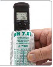
• Calibrate directly in buffer solution sachets
